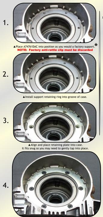
▲ Install 6 allen-head screws and torque to 100-110 inch-pounds (approx. 9ft lbs)
