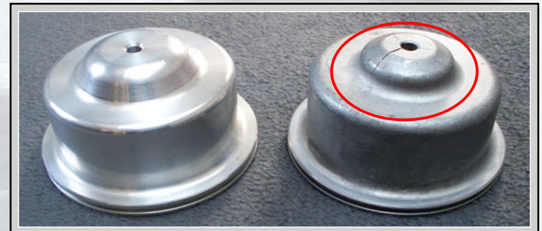
Notice the weakness of the red-circled pin area on the cracked OEM piston compared to the brute strength of our non-porous billet solution.
