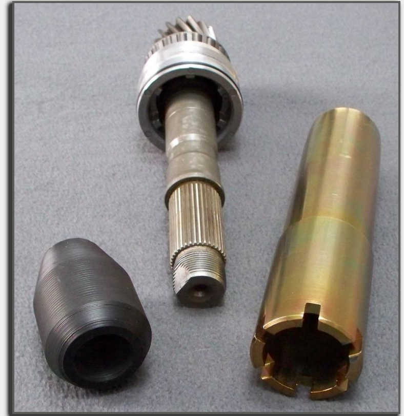
▲ The 2-piece T-7500AC in the foreground with an 01M pinion shaft and threaded support/seal retainer for visual reference.
